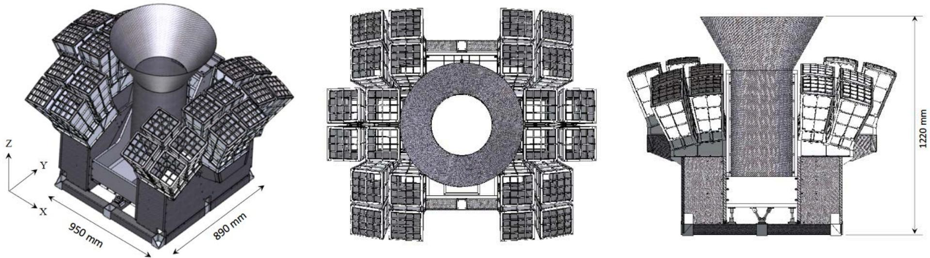
The size of mission payload: 890 mm x 950 mm (base frame) x 1,220 mm (height)
