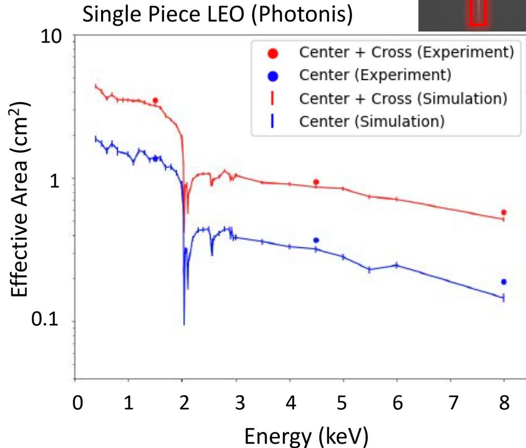
X-ray test at 30 m X-ray beam line
